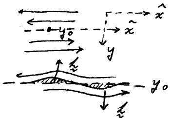
so since  $\Delta v_x/k \sim \omega$ , then  $\omega_0^2 \sim |k v_x|/k$ : in this case, any shear is unconditionally unstable, and the rate of growth is proportional to  $|k v_x|^{1/2}$ , and is fastest for the smallest wavelengths (large  $k$ ).
