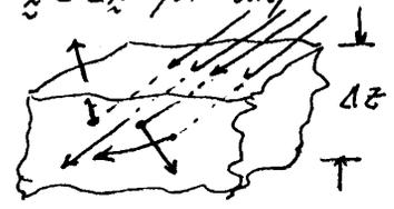
$$\sigma(x, \mu) \equiv \sigma_0(x) p(\mu, \mu') \quad (\text{or } \sigma_0(x) p(\hat{\Omega} \cdot \hat{\Omega}'))$$
