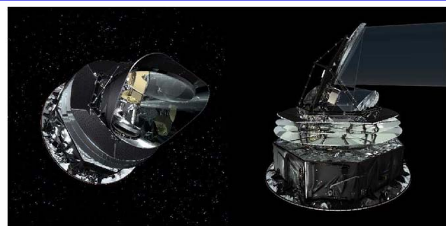
Fig. 4 Two views of a computer model of the Planck spacecraft. The spacecraft spins at 1 rounds per minute (rpm) on an axis normal to the solar panel on the circular end. The spin axis is always within a few degrees of the Sun, maintaining full illumination of the solar panels, at the same time keeping everything else in the dark. This is the first key to the thermal design of Planck .
